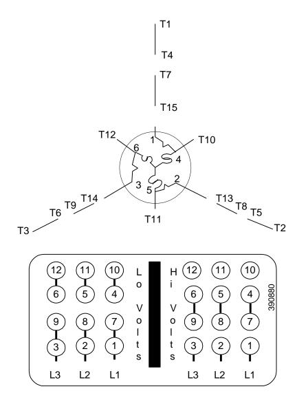
To reverse direction of rotation interchange connections L1 and L2.
