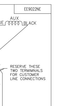
SINGLE VOLTAGE PERMANENT SPLIT CAPACITOR. REVERSIBLE ON TERM. BOARD. WITH OVERLOAD PROTECTION.
