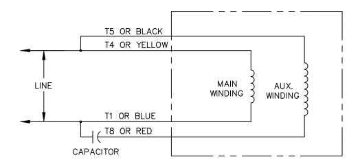
CONNECTIONS SHOWN FOR CCW ROTATION FACING LEAD END. TO REVERSE ROTATION INTERCHANGE T4(YELLOW) AND T1(BLUE) LEADS
