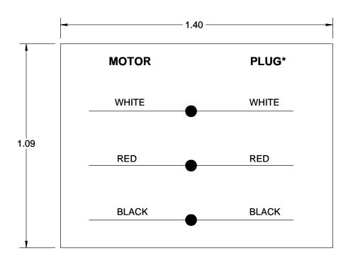
\*NOTE: USE REPLACED MOTOR'S EXISTING PLUG
