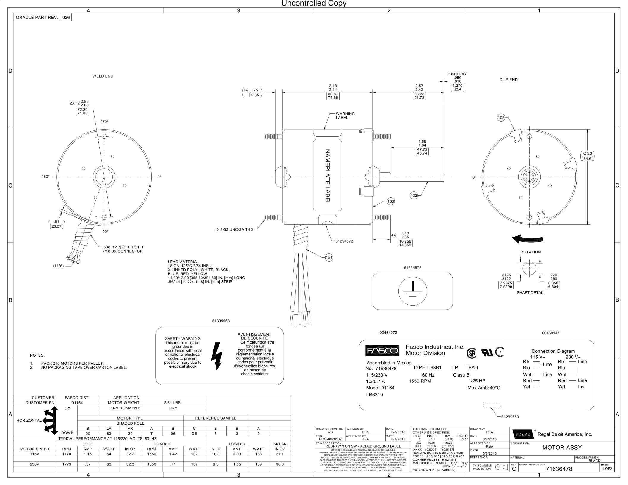
Uncontrolled Copy ORACLE PART REV. 026 NOTES: 1. STAKE STATOR TO SLEEVE PER P.S. 88830264. MAXIMUM TORQUE REQUIRED TO TURN MOTOR SHAFT IS 3/8 INCH-OUNCE. MAKE-UP WASHERS ARE TO BE ADDED OR DELETED TO ACHIEVE REQUIRED ENDPLAY.
