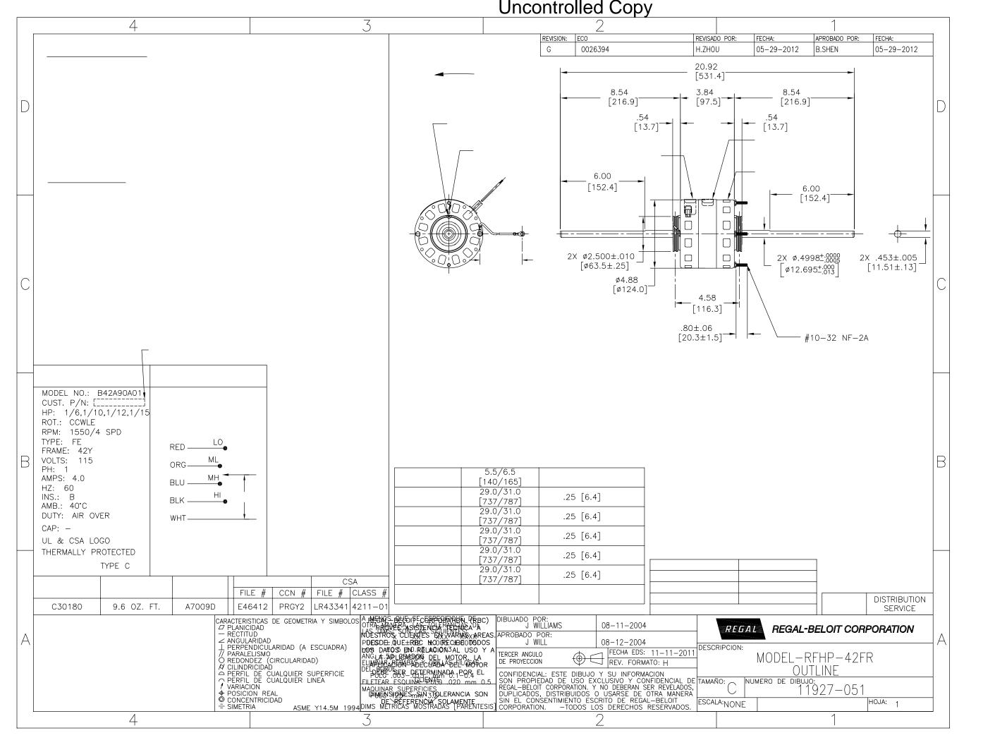
Uncontrolled Copy 4 批准 ECO H.ZHOU 05-29-2012 B.SHEN 05-29-2012 0026394 20.92 [531.4] 8.54 [216.9] 3.84 [97.5] 8.54 [216.9] .54 [13.7]<sup>-</sup> .54 [13.7] 6.00 [152.4] 6.00 [152.4] 2X \(\phi 2.500 \pm .010 \) \(\frac{1}{963.5 \pm .25}\) 2X Ø.4998<sup>+.0000</sup> Ø12.695<sup>+.000</sup> 2X .453±.005 [11.51±.13] ø4.88 [ø124.0] 4.58 [116.3] .80±.06 [20.3±1.5] - #10-32 NF-2A MODEL NO.: B42A90A01 CUST. P/N: [\_\_\_\_\_]
