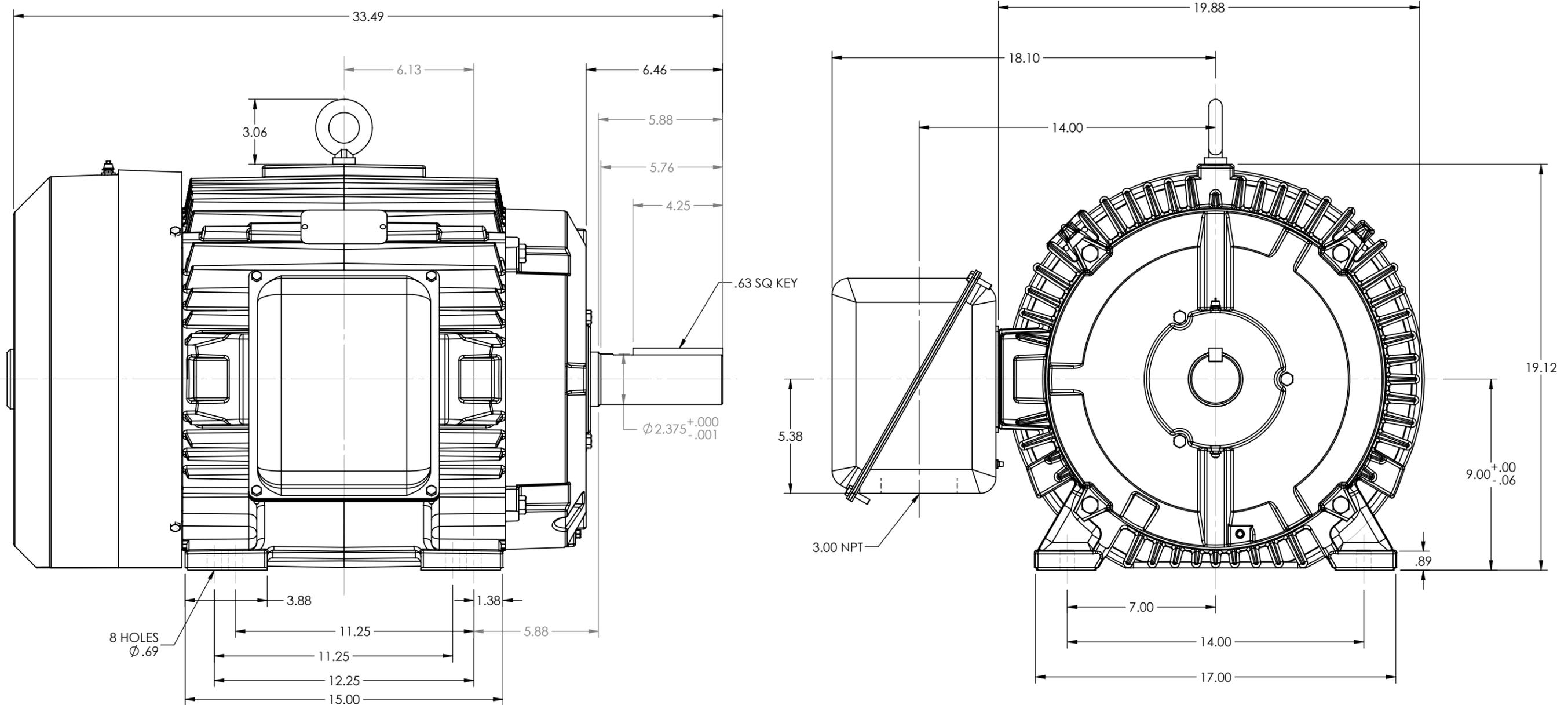
A MAXIMUM PERMISSIBLE SHAFT RUNOUT WHEN MEASURED AT END OF STD. SHAFT EXTENSION IS .002 T.I.R. UP TO AND INCLUDING 1.625 DIA. AND .003 T.I.R. 1.625 DIA. TO 5 INCH DIA.
