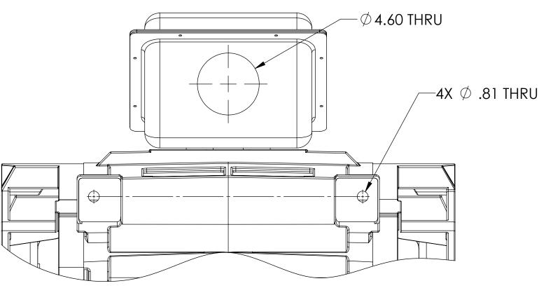
CONDUIT BOX LOCATED ON OPPOSITE SIDE WHEN F-2. IF MOUNTING CLEARANCE DETAILS ARE REQUIRED, CONSULT FACTORY. MAXIMUM PERMISSIBLE SHAFT RUNOUT WHEN MEASURED AT END OF STANDARD SHAFT EXTENSION IS .003" T.I.R.
