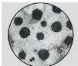
● Material: ductile iron FCD-60.
