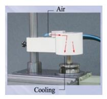
BUILT-IN COOLING FUNCTION The head unit houses both the induction coil and a circular air outlet for cooling air.
