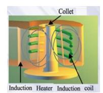
**RAPID HEATING** The eddy current gives out heat from high frequency magnetic field. Shorter cycle time and easy operation.
