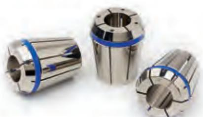
Not only are the slots deburred on all sides, but the collets also have an average roughness depth of the Rz surface area = 1.6 µm
