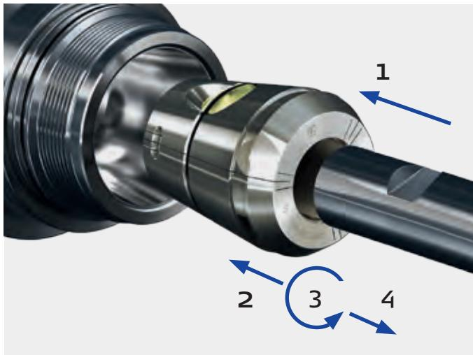
The pin pressure spring is locked in the receptor. The spring applies axial pressure on the tool to preload surface contact between the Weldon and locking wedge.
