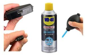
Dirt can get into your connectors when they get unplugged for charging. Issues such as not being able to hear your partner, crackling noises etc may arise. Simply use an air duster or lens duster to give a good blow to clear them out.
