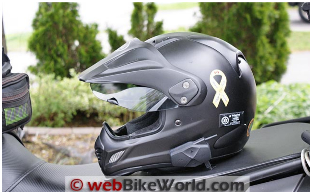
Vertex Raptor-i intercom mounted on Arai XD3.
