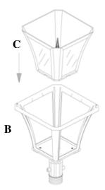
4. Attach top(A) to the body(B) with the two supplied screw caps.
