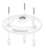
8.2 After assembling attach the three decorative caps provided. and screw the fixture to the base.
