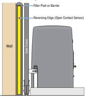
A filler post or barrier may need to be installed between the gate and wall area to reduce the distance to 2 1/4" **or less**. A reversing edge should be installed on the post or barrier for safety (See page 2 for more information).
