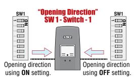
Note: SW 1, Switch 1 - Secondary operator "Opening Direction" will be set the opposite of SW 1, switch 1 on primary operator when using bi-parting gates.
