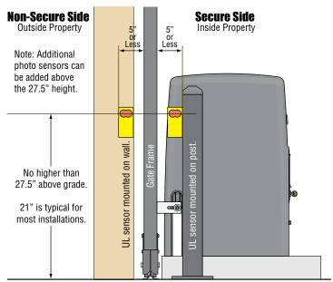
Photo sensors may be installed on either side of gate frame, as close as practical to the gate but no further away than 5".
