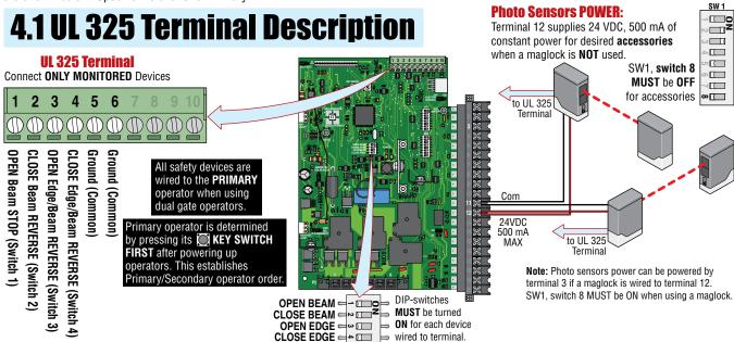
Only 1 monitored Device can be connected to each input.
