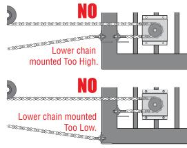
Lower chain **MUST** be 1 inch lower than the endless idler's 180° chain return.
