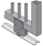
Roller Bearing V-Wheels with Protective Cover - Helps to minimize a pinch point on the gate's wheel and V-rail.
