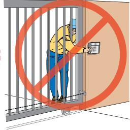
Opening device MUST be mounted a minimum of 6 feet from the gate and NOT accessible through the gate!
