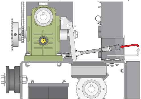
**Manually Push Gate to Desired Position**
