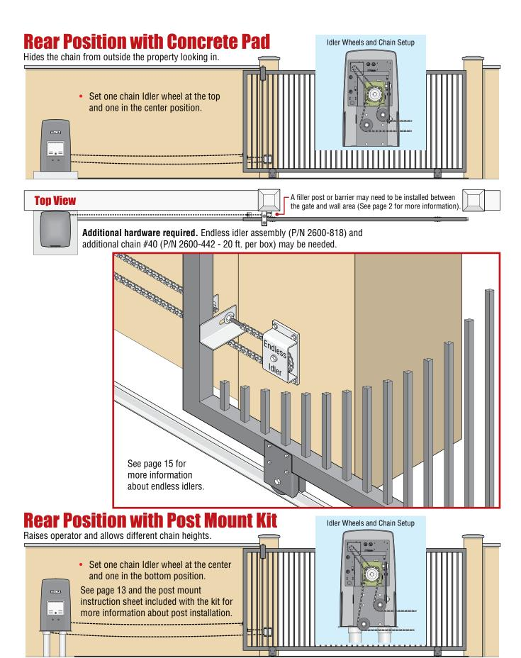
**Additional hardware required.** Post mount kit (P/N 9000-015). Endless idler assembly (P/N 2600-818) and additional chain #40 (P/N 2600-442 - 20 ft. per box) may be needed.
