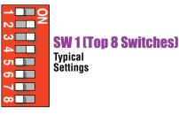
**Switch 1 Must OPEN** the primary operator's gate upon initial AC power up and open command. If the first open command begins to close the gate, turn AC power off and reverse this switch.
