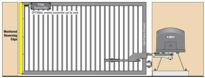
Typical Monitored Reversing Edge mounted on end of gate.
