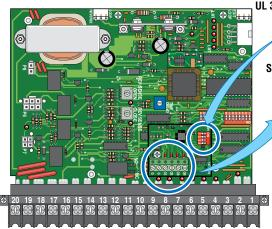
Monitored Device Note: Only 1 monitored Device can be connected to each input. An OPTIONAL Expansion Board (sold separately) will allow connection for additional devices.
