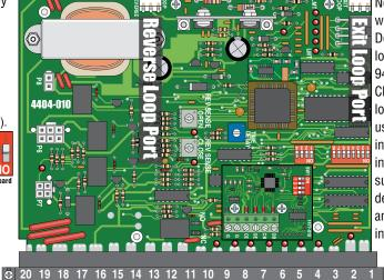
Note: Loop detector wiring is shown for DoorKing plug-in loop detector P/N 9410-010 (Single Channel). If other loop detectors are used, refer to the installation instructions supplied with those detectors for wiring and separate power instructions.
