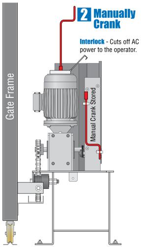
Insert the supplied manual hand crank into the motor shaft underneath the interlock door. Turn the crank to open the gate. Mechanical disc brake on 9555/9556 operator **MUST** also be manually released before manually turning the hand crank.
