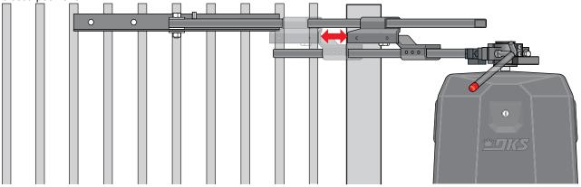
Mark and cut off excess arms. Secure arms to elbow assembly with 6 allen screws. Tighten hub and replace release tool. Install safety covers.
