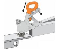
Push handle down and release coupling handle trigger once positioned securely on tow ball. Coupling is now in the locked down position ready for towing.
