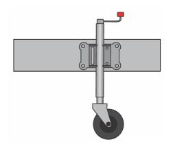
Pull jockey Handle out to rotate Jockey Whee Jockey Wheel/Stand only to be in the vertical position when the trailer is being attached or unattached from the towing vehicle, or in a parked position.
