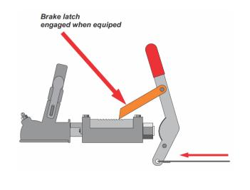
Before unhitching trailer from your vehicle, ensure brake is tightly applied and both wheel chocks (if equipped) are installed downhill of the wheels
