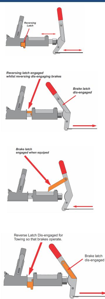
The trailers brakes are operational when the reverse latch is in the OPEN position.
