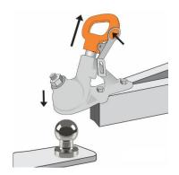
Press coupling handle trigger inwards and pull up the handle to enable the coupling to be attached (or unattached) to the tow ball. USE ONLY A 50MM TOW BALL
