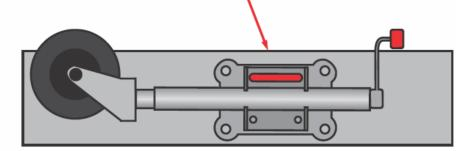
Jockey Wheel/Stand MUST be in the horizontal position with both wheel and handle placed upwards before you commence towing.
