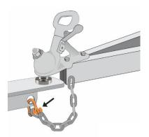
Connect the safety chain/s with D-Shackle/s to the towing vehicle. Cross over chains (if more than one chain) and do not allow to drag on the road.
