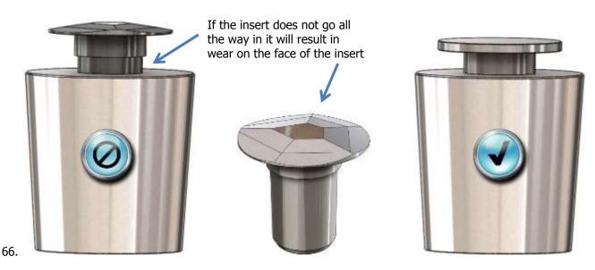
67. Clean out the hole in the plug where the insert goes. Ensure there are no particles or pieces of steel (such as staples ETC). The hole where the insert goes in the plug can be cleaned with a screwdriver to remove packed dust etc.
