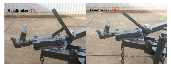
Always ensure the handbrake is off whilst driving or excessive damage to the brakes may occur.
