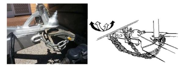
Double back excess chain to prevent dragging. Two chains are crossed under the tow ball to catch the coupling if the trailer disconnects.
