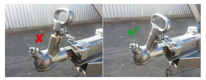
Ensure the coupling locking latch is in the locked position or the trailer will bounce off the tow ball whilst driving.
