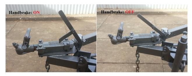
Always ensure the handbrake is off whilst driving or excessive damage to the brakes may occur.
