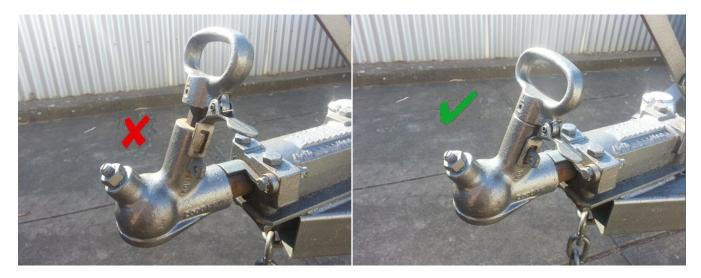
Ensure the coupling locking latch is in the locked position or the trailer will bounce off the tow ball whilst driving.
