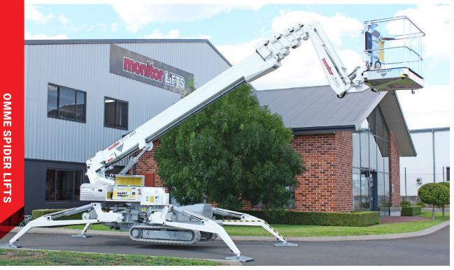
This 31 m Spider Lift weighs only just over 4 t which means it is very suited for use on load-limited flooring. It also makes transport very economical. Variable position stabiliser legs and compact dimensions allow it to set up and operate almost anywhere.
