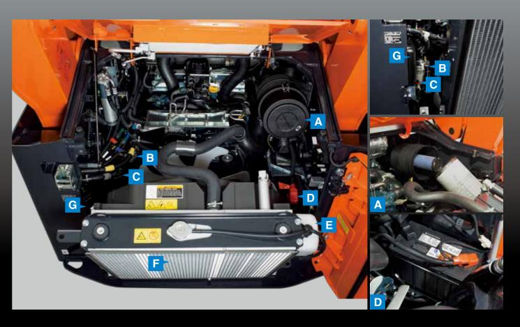
A. Dual Element Air Cleaner **B.** Fuel Filter
