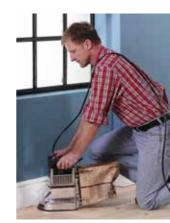
**TIP:** You must hold your thumb on the switch to operate. If you release pressure on the switch it will automatically return to the OFF position.
