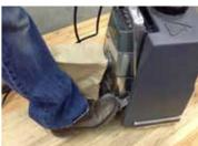
To fit an abrasive sheet make sure the handle is locked in the upright position and tip the sander backwards to ensure it rests on the dust bag frame. The Red or Maroon Abrasive pad must be fitted to the machine. If it looks worn or damaged it must be replaced.
