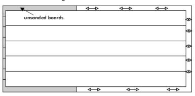
Plank and Strip Floors - sand in the direction the boards are laid, with the wood grain.
