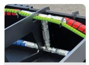
Hydraulic run down protection - anti-cavitation valve
