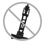
Do not depend on the tilt alarm as a level indicator. The tilt alarm sounds on the chassis only when the machine is on a severe slope.
