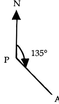
To measure bearings, turn the MATHOMAT upside down and align  $0^\circ$  on the protractor with north on the map. Although now 'back to front' the protractor scale is still easy to use.
