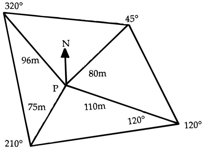
A block of land with corners at A, B, C and D: Bearings and distances are displayed
