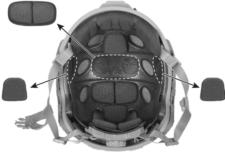
When using the helmet with a communications headset, remove the pads in the center channel of the Vented Lux Liner to allow room for the headset's headband.
