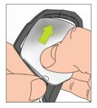
While the frame is open, install the lens by sliding it in towards the outside edge of the frame.
