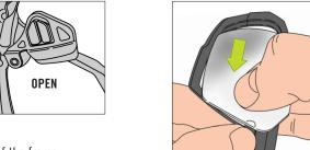
STEP 2 Remove the lens by pulling it towards the center of the frame.
