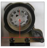
To attach compass, insert light switch into hole. Reattach screws. Red reference line should be perpendicular to individual when in use.
