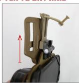
Slide GRT Belt adapter onto GRT rail from the bottom up.
