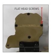
To remove compass, remove 4 screws on the back of the Boltaron platform\*
