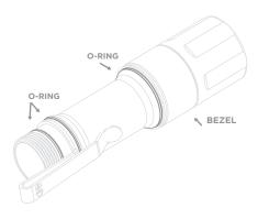
The o-rings on either side of the body: like all o-rings, can and will eventually fail. To prolong their life, periodically apply a small amount of non-petroleum based lubricant. Replacement o-rings can be purchased through www.clouddefensive.com
