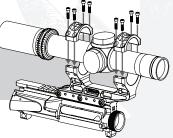
Level scope reticle. Tighten Ring Cap Screws in the order shown, with T15 drive bit. Lightly snug all screws before applying final torque to any screws. TORQUE IN THE PATTERN BELOW TO 18 IN-LBS. COMPLETE THIS PATTERN TWO TIMES. DO NOT USE THREAD LOCKING COMPOUND.
