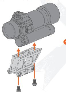
Secure screws using a T25 bit driver.
