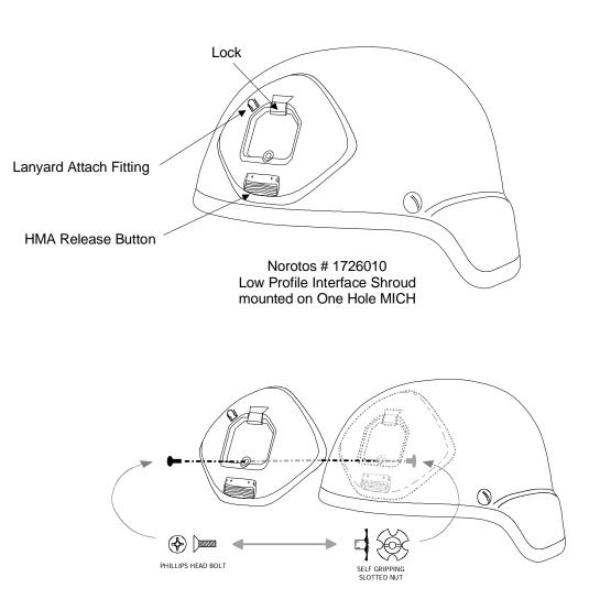
Installation of Low Profile Interface Shroud
