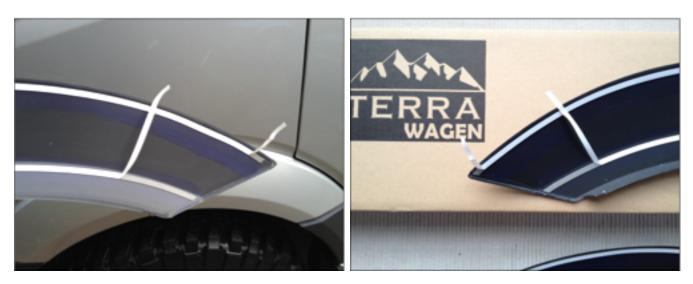
Step 3. Carefully position the fender flare on the fender. While maintaining light pressure, peel the vinyl backing away starting with the center tabs shown in image below. Apply 30 PSI to the taped areas after vinyl backing for the tape has been removed. Note: tape reaches maximum bond after 24 hours of contact.
