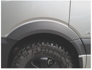
Step 2. Notice that there are 2 adhesive strips, 1 lower, 1 upper. Fold the vinyl backing so that the backing is accessible on top as shown in picture.
