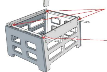
Step 2: Push Metal Frame rest into Frame rest slots.
