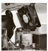
÷ by 13 amps are flawlessly built and finished. Each is equipped with a fan that can be turned off and on to cool the rectifier tube, and the transformers are works of art reminiscent of vintage Woden, Albion and Partridge trannies.
