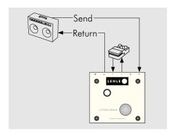
The LITTLE LEHLE III can also be excellently used in FX loops of amplifiers to loop in pedals or even 19"-effects.
