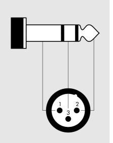
Balanced signal lines are fitted with XLR connectors or TRS (Tip Ring Sleeve) jack plugs. In a balanced signal line, the signal is present in phase at the tip, as in the case of an unbalanced signal line (XLR Pin 2). The second signal conductor carries the same signal, but with the opposite polarity or mirror-image phase (Ring, XLR Pin 3). The third conductor is the screening, and again constitutes the signal ground (Sleeve, XLR Pin 1).
