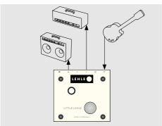
The LITTLE LEHLE III can be extremely useful for switching, when playing live with two amps, for instance, between the clean sound of amp A and the distorted sound of amp B. It also enables you to switch quickly between familiar sounds, or to compare A and B, when you are in
