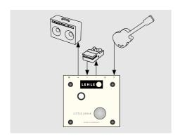
You can use the LITTLE LEHLE III as an effects loop switcher for individual effects units, and also for complete pedal boards.
