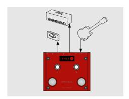
In smaller setups with only 1 guitar and 1 amplifier the LEHLE LITTLE DUAL II can also be helpful to mute the signal for tuning in case you would like to keep it silent for the audience or your fellow musicians. This way the tuner is not in the direct signal path and is isolated electrically from your amp.
