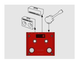
Some instruments are equipped with 2 different type of pickups, usually one magnetic e-guitar pickup and one piezo pickup. These signals have totally different characteristics and sound best when played through their respective amptypes. Usually the instrument offers a TRS jack for the two signals, you can use a TRS-TRS stereo cable. In this case the TRS switch (1) has to be pressed.
