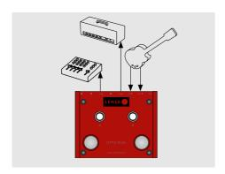
In order to extend the previous setup and to make it more flexible, you can route the piezo signal to a mixer, stage box or DAW instead of a regular guitar amp. This way acoustic and electric guitar sounds can be mixed together, either live for the FOH mix, monitoring or recording. Having the option to convert unbalanced signals to balanced is extremely useful and makes the use of additional equipment like DI boxes redundant.
