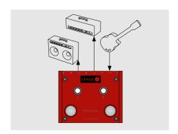
The LEHLE LITTLE DUAL II was designed specifically to split and switch the signal of your instrument between 2 amps which are running at the same time. This way you can achieve very nice blends, e.g. with a clean and a crunchy amp sound. Phasing issues can be corrected at the push of a button, as mentioned previously output A features a phase-inverter switch.
