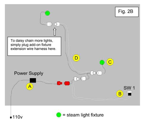
Wiring Tips: To conserve energy when steam room lighting kit is not being used for extended periods, connect the power supply 110v plug into a switched outlet.
