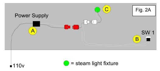
Steam Room Lighting Starter Kit (1 fixture configuration) includes items A, B and C plus 1 LED bulb.
