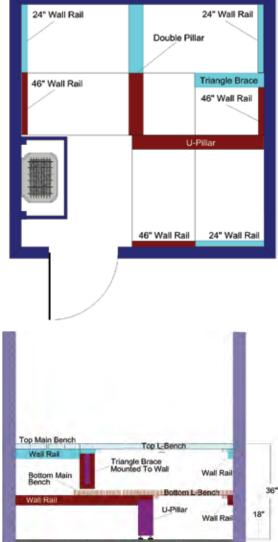
Diagram above illustrates the front view of the installed pillars, rails, and benches on the right side wall.
