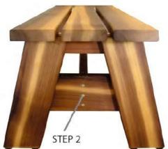
**Step 2:** Align crossmember to leg supports, A to A and B to B with arrow pointing towards top of bench. Fasten with screws into pre-drilled holes.
