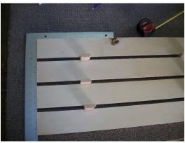
Step 3) Use tape measure and mark two lines top and bottom of each end inset 3/4". Then place lateral support pieces using the lines on each end to align support pieces.
