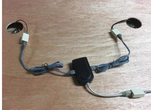
Connect the output cable from the touch control to the male plug on the 8-port splitter via the RJ45 in-line connectors. Once this is done, any of the 8 open ports on the splitter are “live” and can be connected to the RGBW LED light bulbs using the shorter (1 & 2 meter cables) provided in your kit. Any extra cable can be simply rolled up and secured with a twist-tie.
