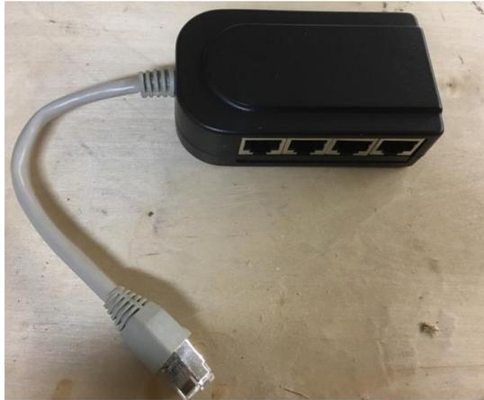
Your kit includes one 8-port splitter with RJ45 connections. You can connect up to 8 LED light bulbs to your system using this splitter.
