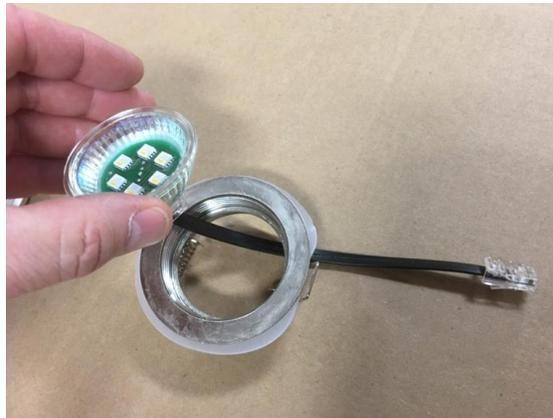
Insert one of the LED bulbs into the front of the housing and screw the lens assembly back in place to secure the bulb.
