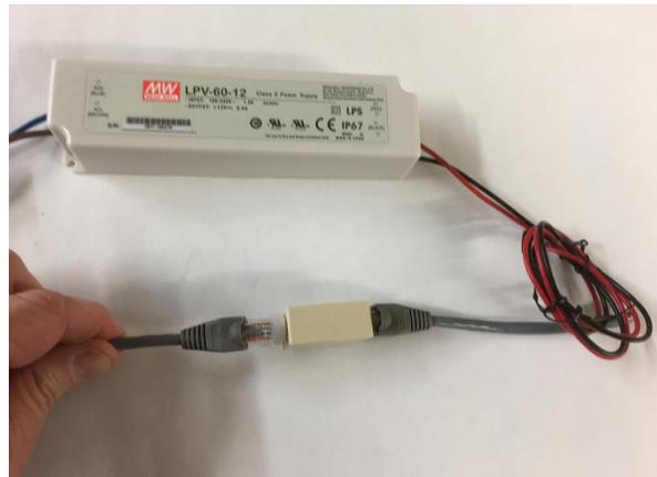
Next, connect the 12vdc input cable from the touch control to the 12vdc transformer using the same method as described above. The black and red wires from the transformer will need to be connected to a constant 120vac/15amp power source. Once this is done, you should have completely functional LED lighting system.
