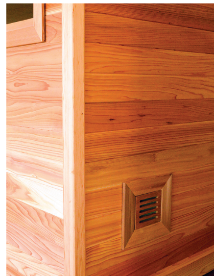
Outside view of installed Sauna Vent Kit. Inlet vent should be under Sauna Heater as shown here, to heat incoming air.
