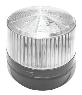
Model OE-STROBERPC is a high output, rainproof strobe suitable for both indoor and outdoor applications. Strobe life expectancy is 50,000 hours, up to 250 times that of comparable models. Mounts on bell box or other enclosure (including W Box model OE-STSTSIREN) or directly to wood or other surface. Two bolts, two nuts and two wood screws are provided. An adhesive mounting gasket is provided to enhance rainproofing. A rubber ring seals the lens with the base.
