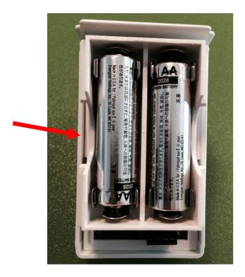
Tech Tip: Carefully notch the plastic housing to allow the back plate to slide back on and close properly.
