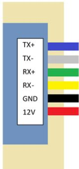
The other end of these wires connect to similarly labeled terminals on the gateway inside the communicator box, but the order of the wires is switched. *TX+* and *TX-* on the communicator remote mounting module should connect to *RX+* and *RX-* on the gateway, respectively. Likewise, *RX+* and *RX-* on the communicator remote mounting module should connect to *TX+* and *TX-* on the gateway, respectively. The GND and 12V wires should not be switched.
